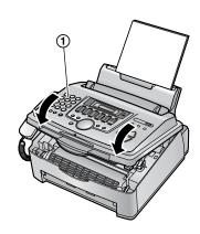
While the unit displays "PLEASE WAIT", do not open the front cover, or disconnect the power cord.
